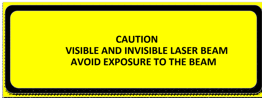
Explanation Label Figure 2 of AS/NZS IEC 60825.1:2014 Showing possible alternative wording Detailed dimensions for this label are contained in AS/NZS IEC 60825.1:2014
